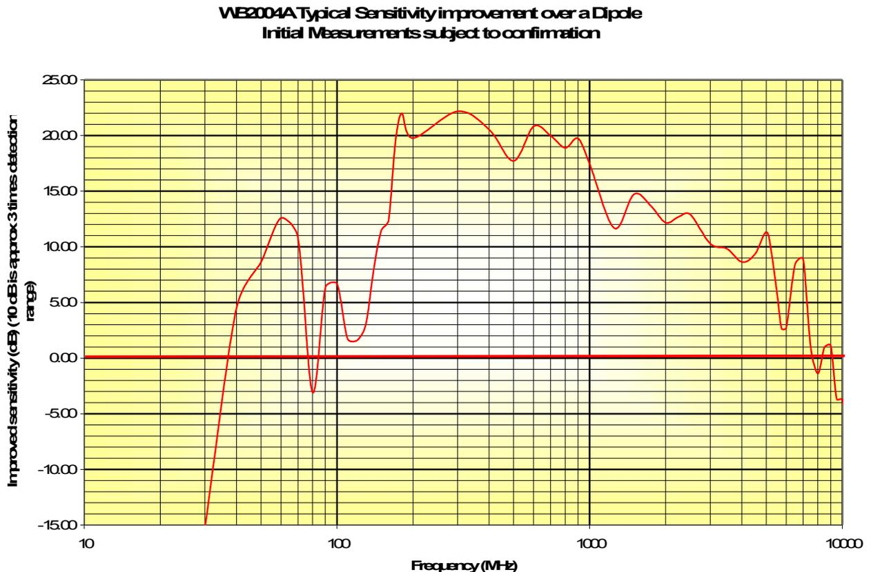
10 dB improvement is three times the detection range, 20 dB is ten times the detection range.
